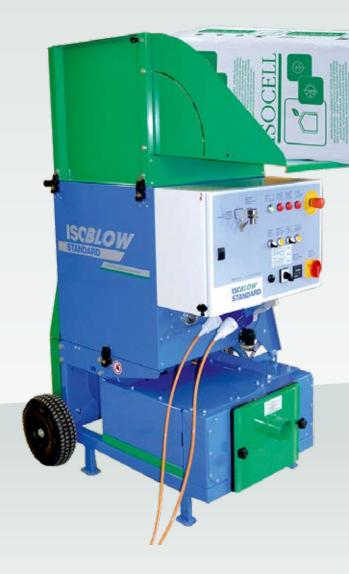
The ISOblow STANDARD is a very powerful extraction in combination with ISOCELL blowing machine for the processing of cellulose insulation as well as other approved loose and free-flowing insulation materials. The filling is carried out via a filling flap. The attachment can be removed for transport. Two shredder shafts in the lower area of the hopper ensure very good loosening of the cellulose. The ISOblow STANDARD is operated and the material
