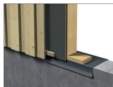
D7. Transition between walls
